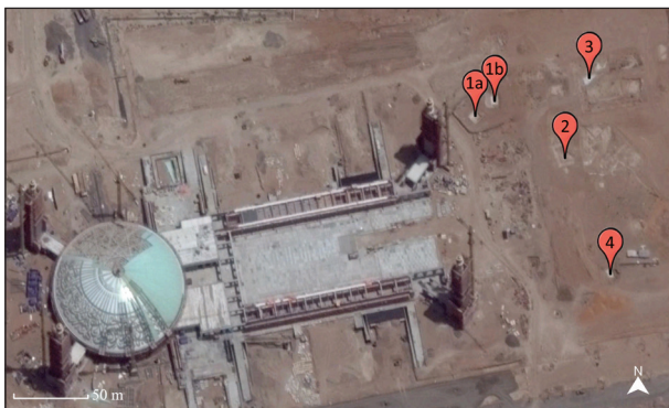
Fig. 5: Location of the preserved architectural units in relation to Sheikh Khalifa Grand Mosque. Unit 1a is a short stretch of Falaj 1, Unit 1b is the Mosque, Unit 2 is Building 1, Unit 3 is Building 4, Unit 4 is a thugba (shaft hole) on Falaj 1. Google Earth image 2018.
