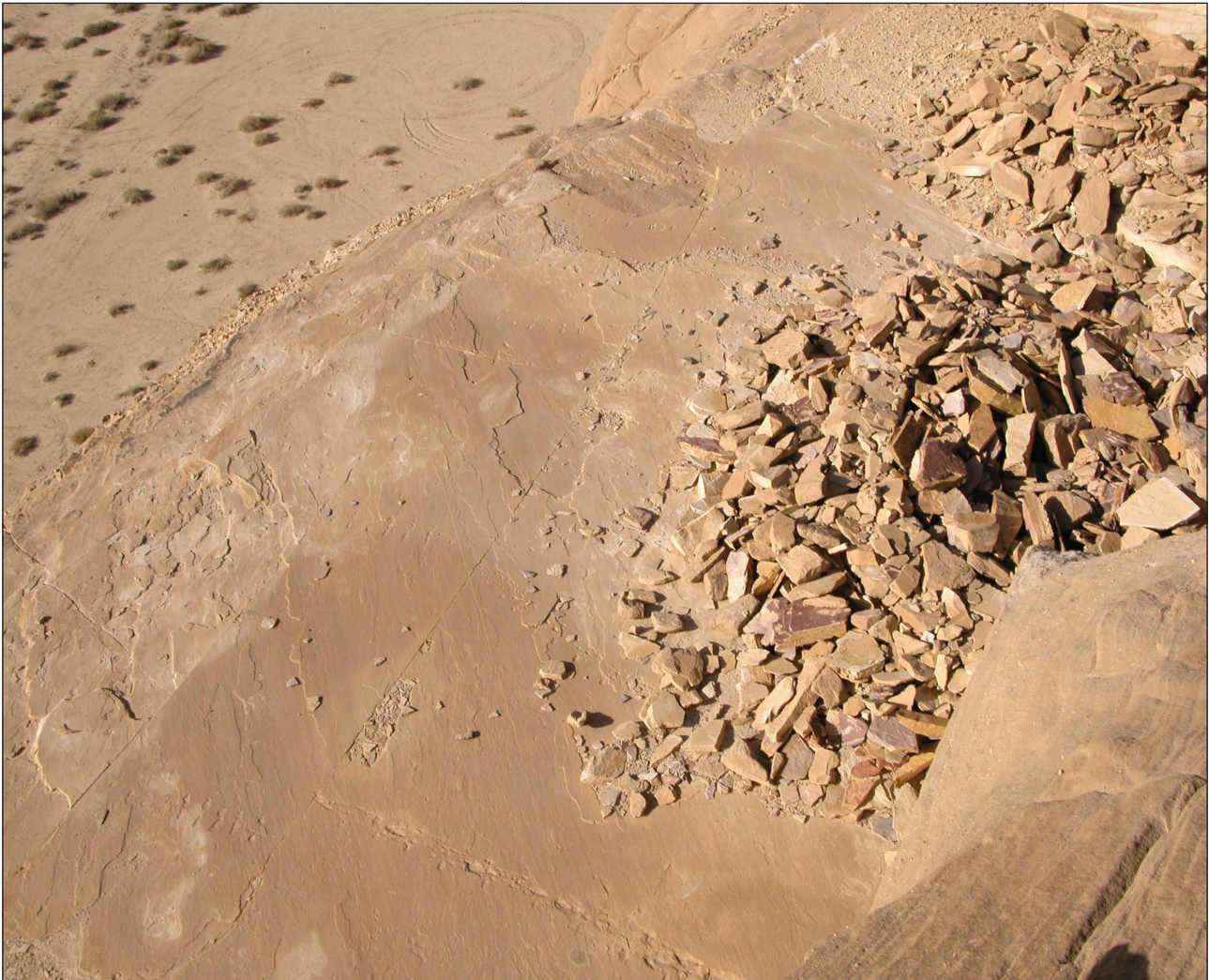
Fig. 2. Probable ancient quarry Mah28. Note the traces of the wedges on the terrace.
